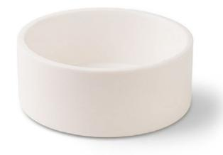
Resealable jar made in Mullite and designed to obtain correct and homogeneous firing of the Zirconia, also protecting it from discoloration which occurs during sintering.
