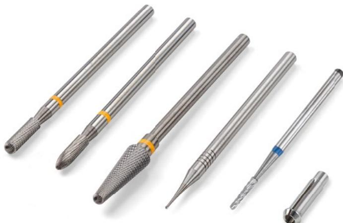
Kit designed and created to allow the technician to work the Zirconia after sintering. Dedicated tools allow you to obtain the best technical and aesthetic results in this delicate and very important phase of your work.
